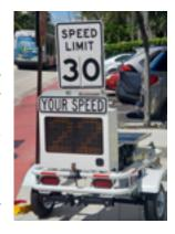
reports detailing dates, times, speeds and volume. The trailer is easily deployed and repositioned throughout the community for maximum effectiveness. It operates continuously for up to seven days and is equipped with a solar panel for extended operation.
